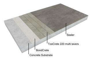
Installation on Tiled Floor or Concrete w/Cracks
